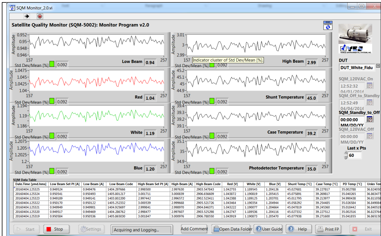
Figure SS5. During execution, the lamp currents, internal temperatures, and photodiode signals are graphed, and the data is displayed in tabular form. The operator would have selected the current DUT from the pull down menu and set the time the AC power was activated and the rotary knob was switched from “off” to “standby”. In real time, the operator can change the number of points being averaged, which is used to determine the relative percent standard deviation for each data stream. The colors of the green squares go from red to yellow to green depending on the relative percent standard deviation.
