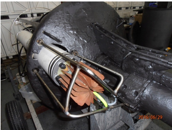
Figure 28) New blue spectrometer installed on side of MOBY Heritage buoy. To operate in this manner we have additional collectors installed alongside the normal MOBY collectors as shown in Fig. 29.
