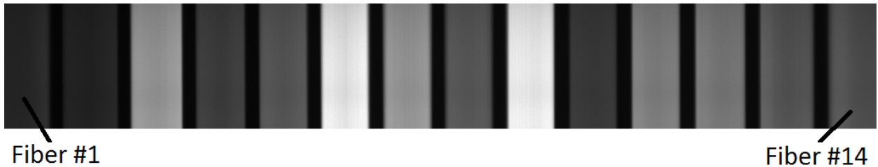
Figure 14) Fiber 1 and Fiber 14 (tracks 1 and 14) are not imaged totally on the array.
