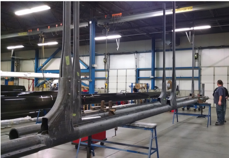
Figure 26) MOBY-Net carbon fiber spar and arm assembly.
